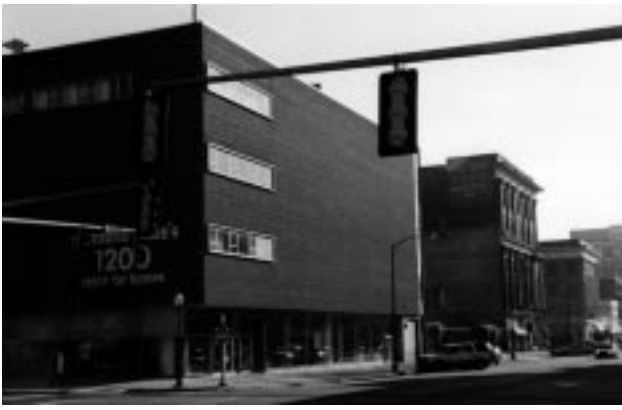
The building in the foreground is not a good example of new construction in the downtown area; it lacks the appropriate scale, width, and rhythms of architectural details and openings.
