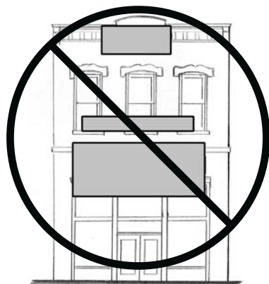
Fig. 4.1: INAPPROPRIATE Sign Placement
